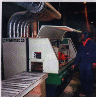
Foreman Kiko Reece uses the company's Weinig Profimat P23 five-head moulder, one of its first major machine purchases.
