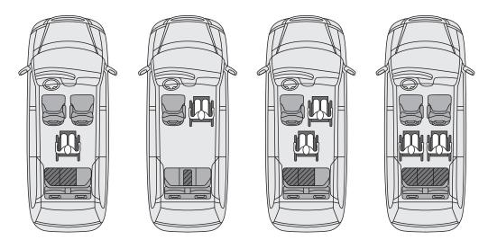
Wheelchair users cannot drive from their wheelchair in the Northstar E conversion because the front driver seat is not removable. Seating options may vary based on available payload. Refer to your VMI owner's manual for payload information.
