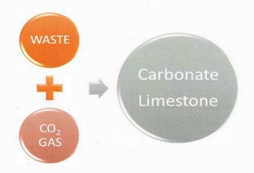
During the process, significant volumes of carbon dioxide are permanently captured. Not only does this help with the binding of the materials, but importantly chemically stabilises and encapsulates contaminants.
