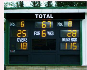
Having visited the site, ESU provided drawings and instructions to enable the club's carpenter to make the necessary modifications. ESU constructed windows faced with anti-glare polycarbonate which were then fitted to the newly painted fascia and with the LED digits installed and signboards erected the scoreboard was completely transformed.
