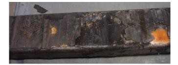
Figure 3a: Observation of the degradation of the semicon coating of Bar L3-1 from Machine 5 (a motor-generator), which had the lowest PDEV and the highest PD magnitudes. This image also shows local burning and PD attack on the bar surface.
