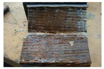
Figure 3b: Burning and PD attack between the groundwall and the copper stack. The green areas are where the PD has corroded the bare copper strands (half the strands were not insulated in this machine).
