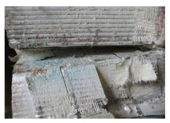
Figure 2: View of turn insulation and conductor stack of coil LC1 from Machine 6. Note that the delamination at the turn resulted in heavy partial discharge attack that further damaged the turn insulation. The green powder is from oxidation of the copper by ozone from the PD.
