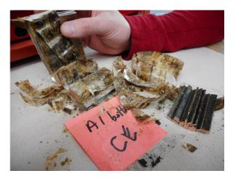
Figure 1: Photographs from the dissection of a segment from Coil A1 from Machine 1. Machine 1 had seen 56 years of base-load operation, but did not experience an in-service failure. Once the axial cut through the groundwall was made, the turns and strands from Coil A1, slot exit (connection end) fell apart. The turn insulation was burned and there was extensive PD attack.
