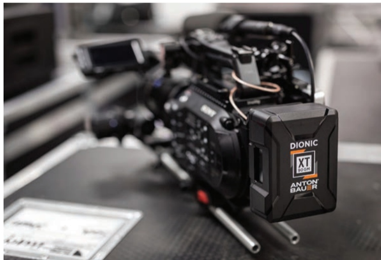
Dionic XT from Vitec Group's Anton/Bauer is a 14V Li-Ion battery capable of delivering up to 12A of continuous power.
