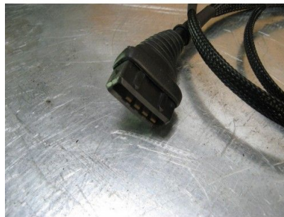
Plug and play wiring loom AFM connector
