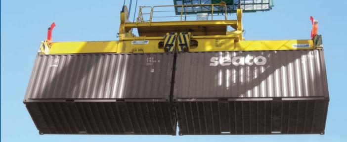
The RAM 2900 series Twinlift CenterSpread has been developed to provide productive, safe and cost-effective container handling for both ship-to-shore cranes and yard stacking cranes. The versatile Twinlift concept allows the crane operator to lift a 20', 40' or 45' container, or two 20' containers at once, all with the same spreader unit.
