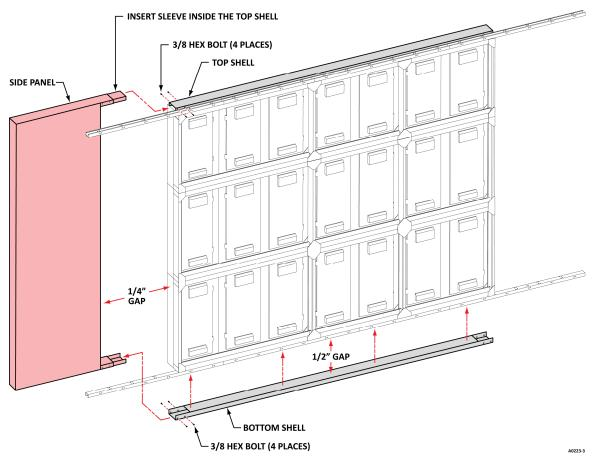
FIGURE 16 – SIDE PANEL TO TLVISION SECTION
