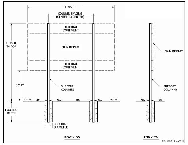
FIGURE 2 — TYPICAL SUPPORT COLUMN STRUCTURE
