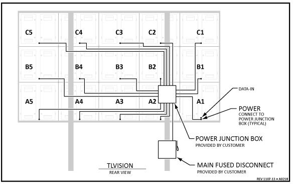
FIGURE 22 — POWER CABLE CONNECTIONS
