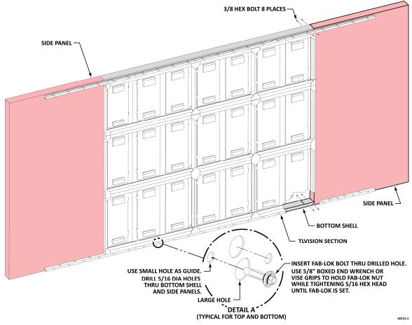
FIGURE 17 - INSTALL SIDE PANELS TO TLVISION SECTION
