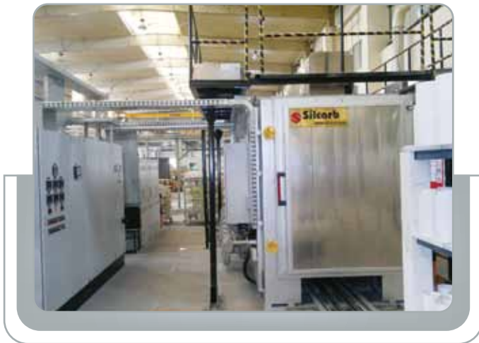
1550° C TWO CAR KILN INSTALLATION FOR CERAMIC GLAZING, WITH CONTROLLED COOLING
