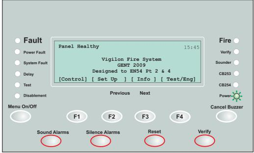
The **MENU ON/OFF** button facilitates the operation of the function keys F1 to F4. The menu prompts appear on the display above the function keys to prompt the user to make a selection.
