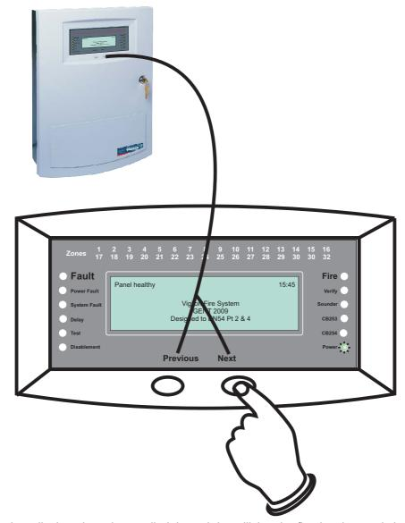
The FIRE events when displayed can be scrolled through by utilising the first level controls located as shown on the panel front door.
