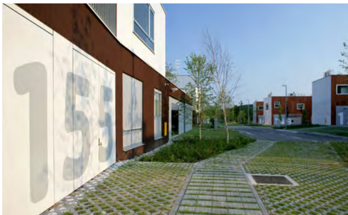
Figure 3.15 Permeable surfaces and open grid pavement patterns are encouraged wherever possible in the neighbourhood, including private laneways
