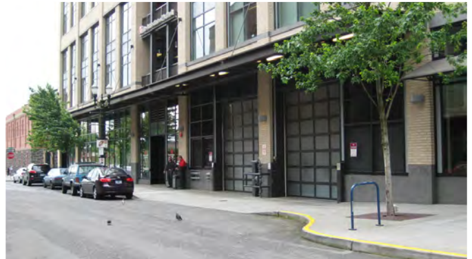
Figure 3.20 Access to servicing and parking treated as a part of general architectural wall design.
