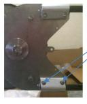
Loosen the clamping nuts
