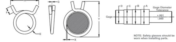
**EFFECTIVE CLAMPING RANGE:** After expanding to no greater than "A" diameter of the gage, the clamp in relaxed condition shall not pass over "D" diameter. When clamp is assembled on "A", "B" or "C" diameter of gage, a wire of "X" diameter shall not pass between gage and clamp when inserted in a direction parallel to the axis of the gage.
