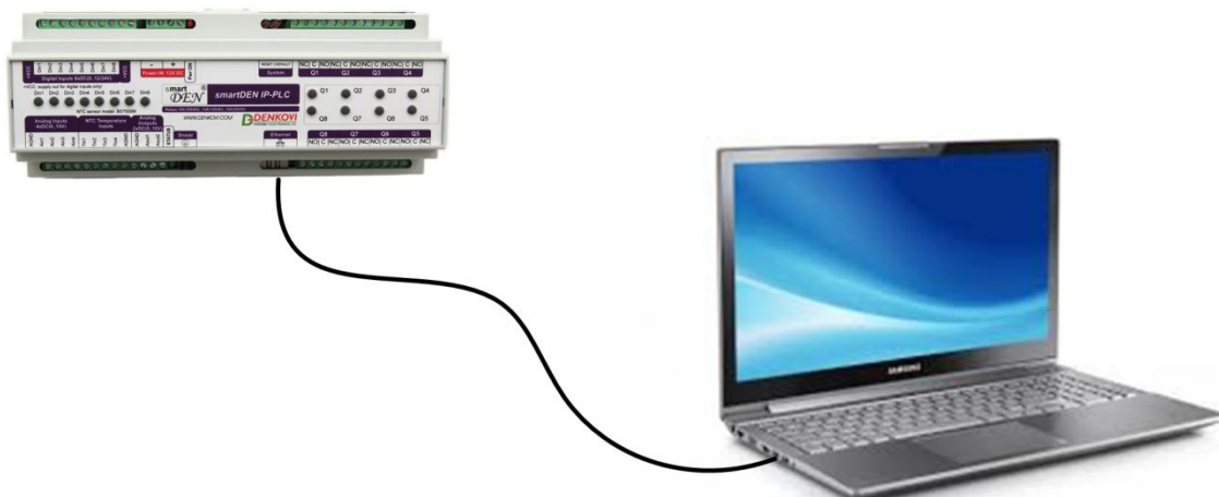
Figure 5.10. Direct connection of smartDEN IP-PLC to a computer
