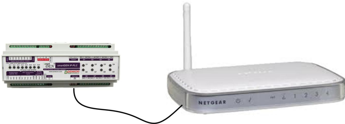
Figure 5.11. Connecting smartDEN IP-PLC to a wireless router
