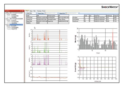
Interface with your ShockLog device through a simple Windows®-based software program. Clear instructions allow for quick deployment and easy data analysis. The ShockLog Report View provides an overview of the entire journey. Zoom in for a closer view, or export data into programs such as Excel and MatLab for more detailed analysis.
