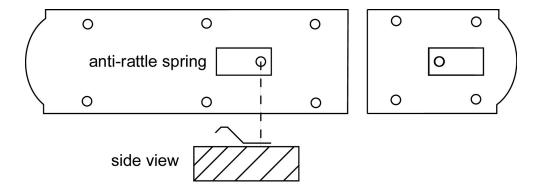
4. Drill 1/16" pilot holes at the locations you marked for the bolt and catch. Place the bolt and catch over the springs and screw them to the shutters. Test the operation.
