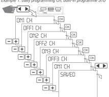
1. Press the **SELECT** • until indicator lamp **PROG** is ON.
