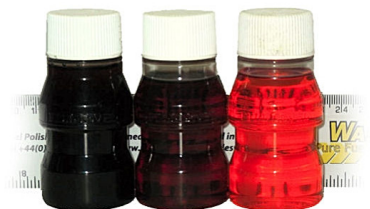
Left to right, before fuel cleaning, after 1st stage, after complete clean
