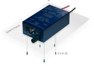
DP03 series probes can be mounted directly on a base plate or enclosure walls with 5 x 6-32 screws. Optional mounting flange models are available, shown below. These can be mounted with 4 x 10-32 (or M5) screws.
