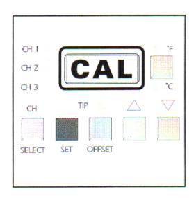
22.Press and release the Tip Temperature Offset Key two times to exit calibration. All values, features and defaults entered during the calibration are now stored in memory and all channel tip temperature settings are turned "OFF". All channel Tip Temperature Offset settings are set to the default value of 6°F (3°C).
