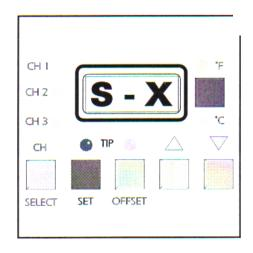
7. Press and release the °F/°C Key to change the default. Each subsequent press and release of the key will change the default
