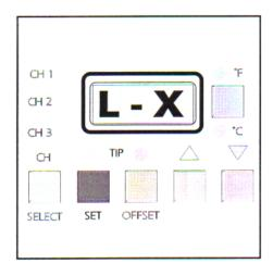
13. Press Scroll Keys as necessary to increase (Scroll Up Key) or decrease (Scroll Down Key) the Lower Temperature Limit value.
