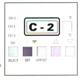
20. Unplug the #1 Calibration Assembly and plug in the #2 Calibration Assembly.
