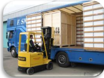
Figure 11 – Fork lifting containers on/off vehicle
