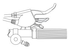
Position bell on left hand or right hand side of the handlebar as required.
