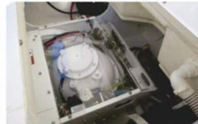
▲ This is the smallest of the units made by US-based Seakeeper, seen here as a boat show demonstrator in an 8m (24ft) sportsboat. IBI tried this unit, the 12V Seakeeper 2, for ourselves, and were impressed with its ease of use and strong damping effect
