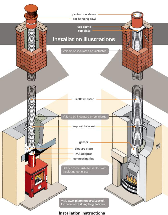
NOTE: For clarity, masonry has been omitted from part of illustrations.
