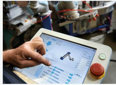
"We opted for the UR5 robot due to its unique features including the robot's ability to stay in the same position even when it is switched off. This is particularly important when using robots for testing the trajectory of hand movements in interventions requiring precision, accuracy, and safety."
