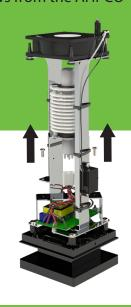
3. Grasp the AHPCO® Cell and pull to the side, then remove the lamp connector.
