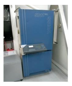
Additionally, our Weiss SBII environmental chamber, with internal dimensions of H26"  $\times$  W21"  $\times$  D16.5", offers a temperature range between +180°C and -40°C, with a ramp rate of approximately 3°C per minute. This chamber provides a 10-98% relative humidity.
