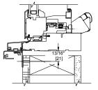
Standard Sill Nose. Add 13/16" (21mm) to Frame Dimension at Sill.
