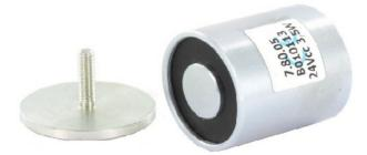
This magnet exerts a holding force POWER OFF, of approximately 15 Kgf perpendicular to the steel catch plate with which it is in contact.
