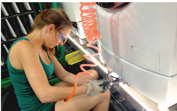
BEFORE: For eight hours a day, the operator looks down into a small mirror with a light shining in her eyes, to see the small holes that she fills with three screws. Her neck is bent and her knees are brushing the line.
