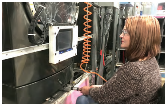
AFTER: Operator looks into the monitor to determine where the screws go. No bent necks, no constant light bothering her eyes, no knees touching the line.
