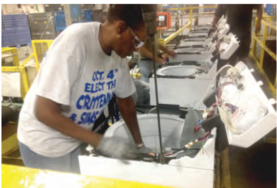
BEFORE: Washing machine assembly put constant stress on workers' back, neck shoulders, elbows, hands and wrists.
