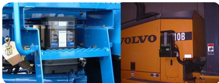
Central Lybrication System unit on the machine
