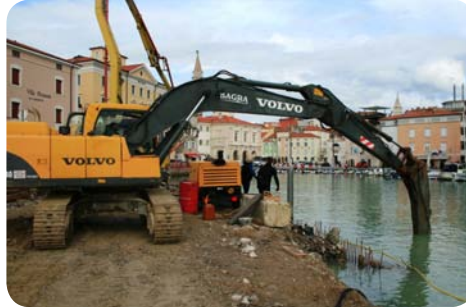
Underwater digging - Arm extension enables digging in positions that are much below excavator level - for example digging in the water (sea, river ...)
