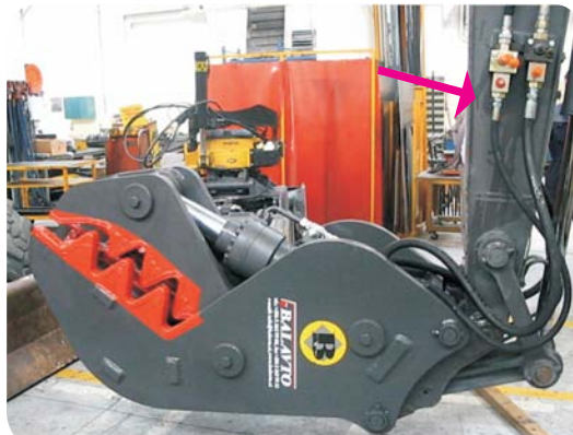
Hydraulic shears hoses attached to the excavator with B-Quick
