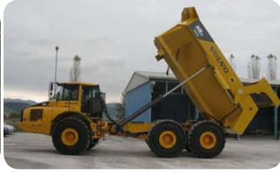
Light material dumper bodies are often used in Termal Power Plants for ash transportation
