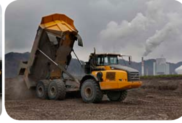
Light material dumper bodies are often used in Termal Power Plants for ash transportation
