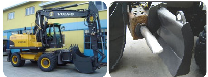
Hydraulic Breaker Carrier positioned on the Blade is an excellent help during the Breaker transportation from one site to another.
