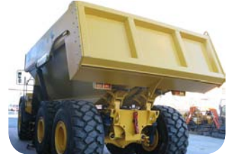
Dumper body can be firmly closed (sealed) so it is also appropriate for liquide materials transportation
