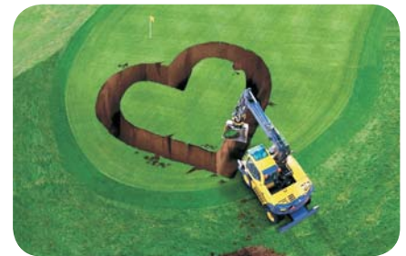
Unlimited rotation and tilting of up to 40° in two directions
