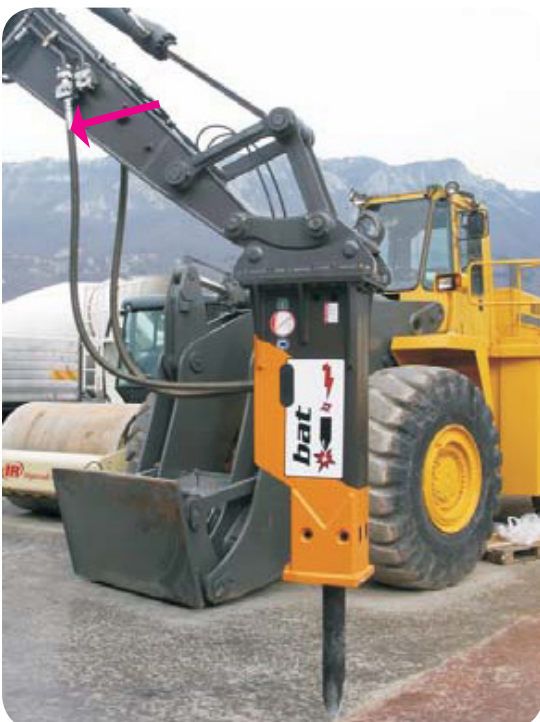
Hydraulic breaker hoses attached to the excavator with B-Quick
