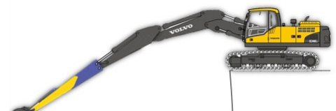
B - Digging reach = 15 m Volvo EC240 with arm extension - Long reach Arm
