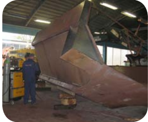
Light material dumper bodies are often used in Termal Power Plants for ash transportation
