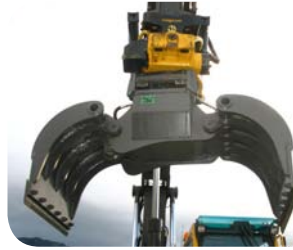
BG 13 without rotator connected to the excavator with Tiltrotator
