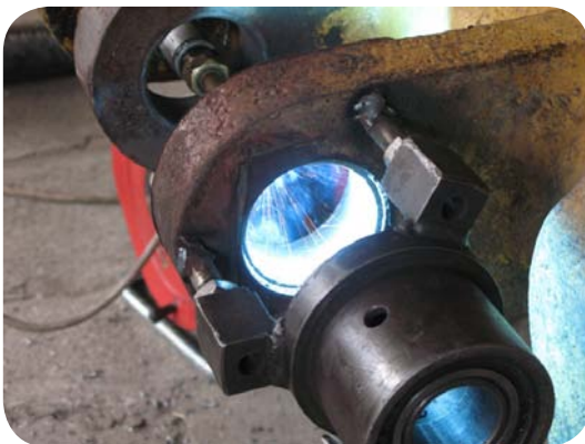
Pins and bushing repairing and mounting them on the machine
