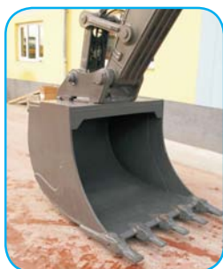
Bucket and Quick fit, both made on Balavto
