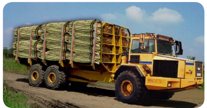
Dumper used for sugar cane transportation
