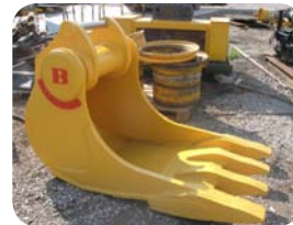
Buckets for stone placing
