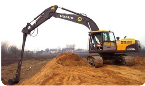
Volvo EC240 with arm extension - Long reach Arm, an excellent tool on site
