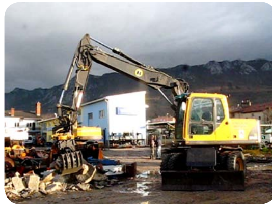
BG 13 without rotator connected to the excavator with Tiltrotator
