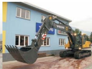
B1 Quick Fit and bucket turned for 180° and connected to the excavator (which enables B1 quick fit)
