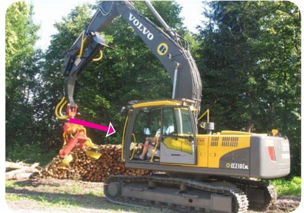
Volvo EC210C excavator with special protecting glass on the cab - made by Balavto Ltd.
