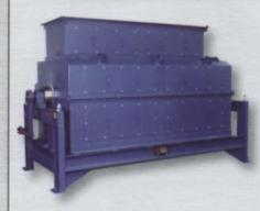
High Speed Permanent Drums are designed to suit specific application requirements and are suitable for the dry separation of highly magnetic ores such as iron ores, nickel ores (magnetite), roasted ilmenite and similar.
