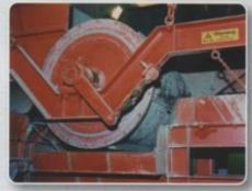
Drums are suited to any continuous processing of material; from the separation of paramagnetics from minerals and powders, to the recovery of ferrous metals from fragmentised end of life vehicles and refuse reclamation.
