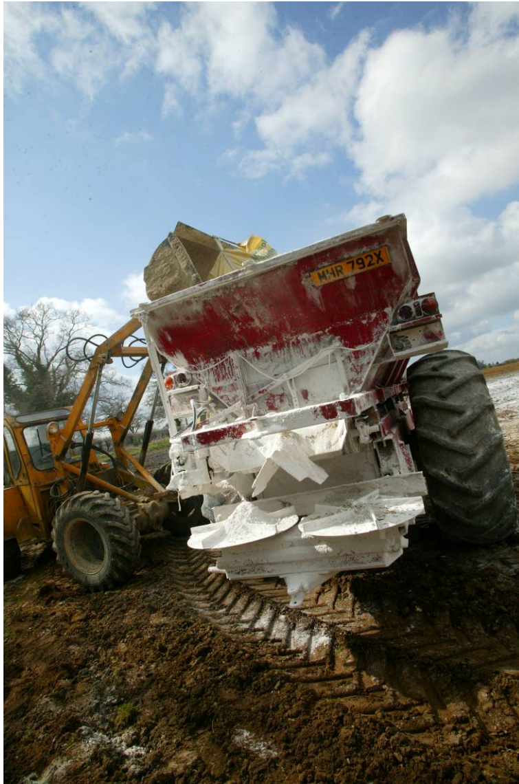
Figure 11 Spreading mechanism of the lime spreader used
