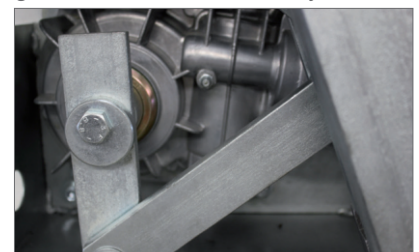
Easy maintenance thanks to the double greasers both on housing and gear motor
