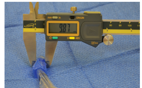
Figure 2: Example of a Shiley 37 Fr Left DLT endobronchial measurement (in mm, this important endo-bronchial diameter is not indicated on the packaging, see Fig. 1).
