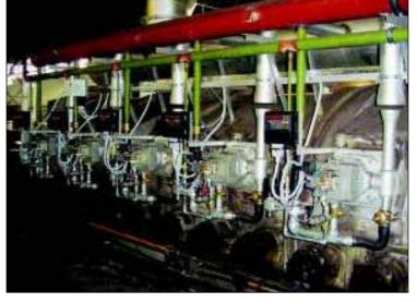
reconstructed gas heated tunel furnace - 5m x 60m - 1300°C
