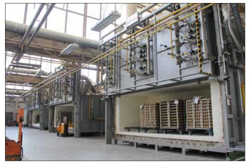
gas heated chamber furnace - 6m³ - 1350°C
