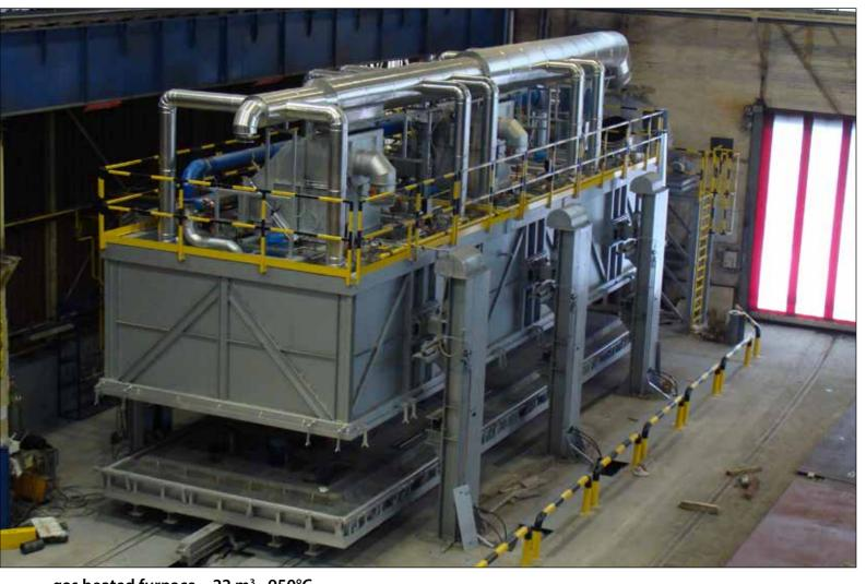
gas heated furnace - 22 m<sup>3</sup> - 950°C
