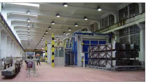
gas heated oven - 12 tons - 250°C
