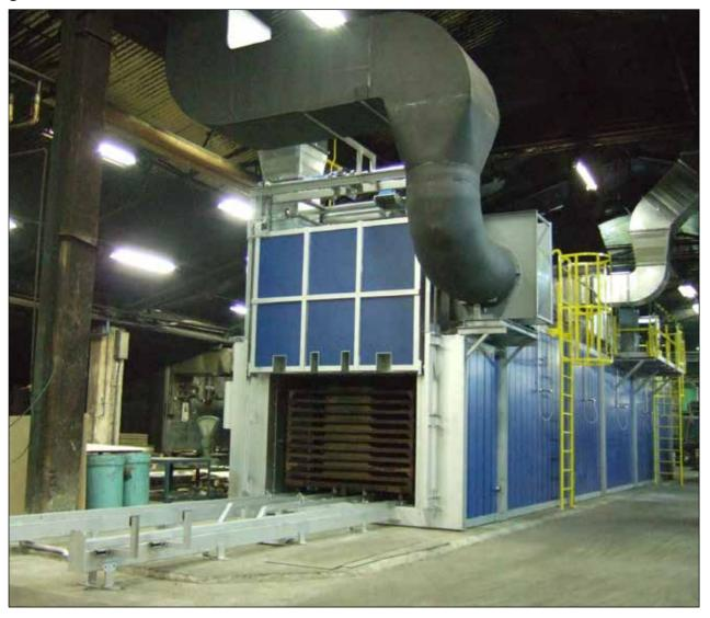
gas heated tunnel furnace
