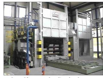
gas heated furnace and cooling chamber -  $20 \, \text{m}^3$  -  $450^{\circ}\text{C}$
