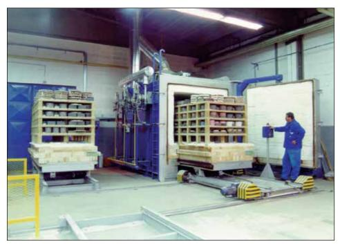
gas heated bogie hearth furnace -  $5m^3$  -  $1300^{\circ}$ C
