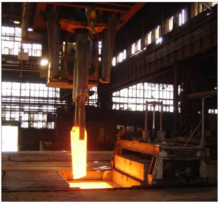
reheating gas heated furnace for ingots
