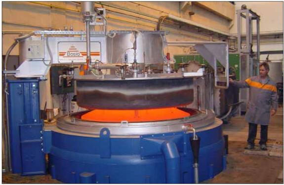
electro heated pit furnace (controled atmosphere) - 9 m<sup>3</sup> - 950°C
