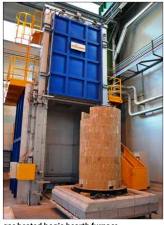
gas heated bogie hearth furnace  $\,$  -  $\,$  12  $m^3$  -  $\,$  300°C
