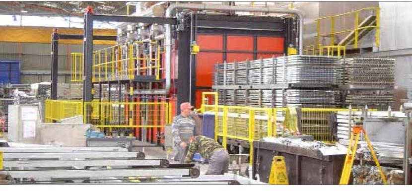
gas heated oven - 15 tons - 250°C
