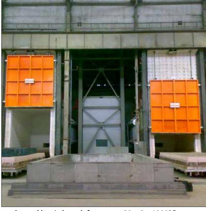
gas heated bogie hearth furnaces - 59 m3 - 1200°C
