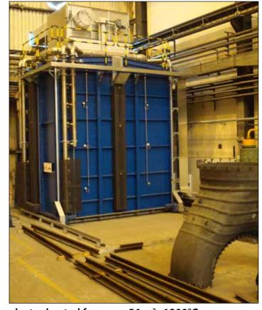
electro heated furnace - 56 m<sup>3</sup> - 1200°C
