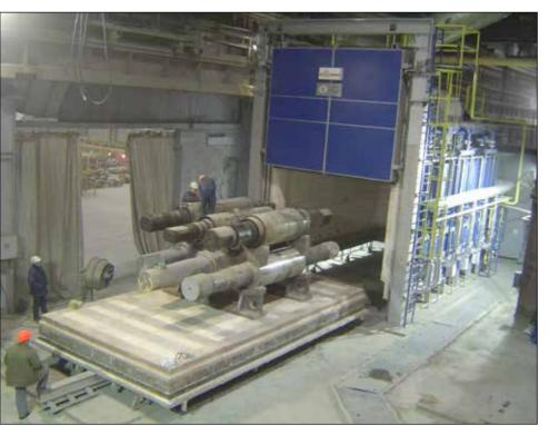
gas heated bogie hearth furnace - 70  $\mathrm{m}^3$  -1200°C
