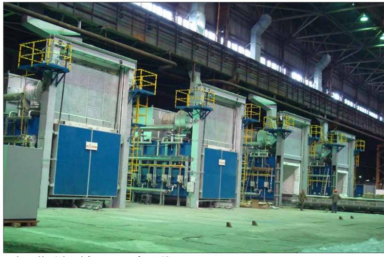
gas heated bogie hearth furnaces - 47  $\,\mathrm{m}^3$ - 1100°C
