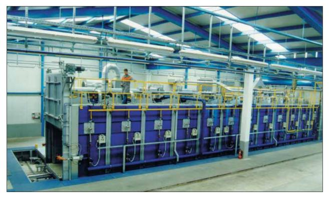
gas heated tunnel furnace -  $12 \times 28 \text{ m} - 250^{\circ}\text{C}$
