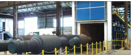
gas heated bogie hearth furnace -112 m<sup>3</sup>- 1150°C
