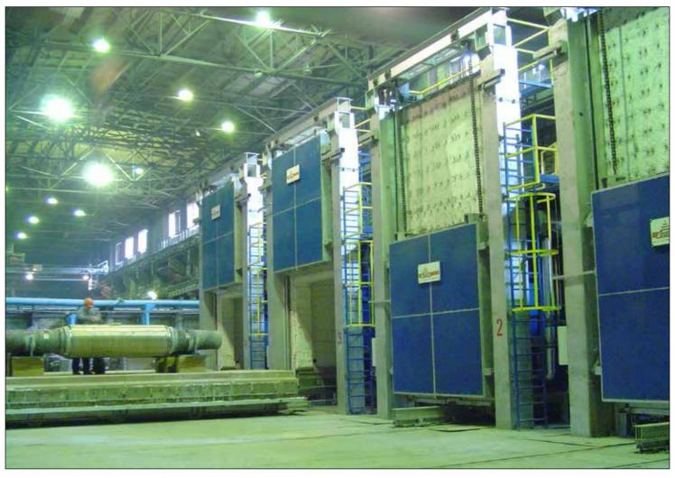
gas heated bogie hearth furnace - 34  $\mathrm{m}^3$  - 1200°C
