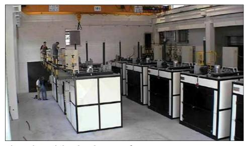
electro heated chamber dryers - 8m³ - 250°C
