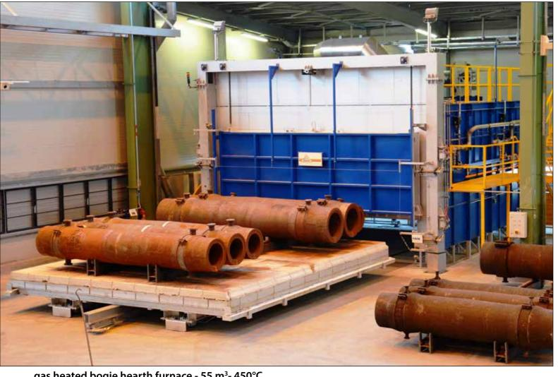
gas heated bogie hearth furnace - 55 m<sup>3</sup>- 450°C
