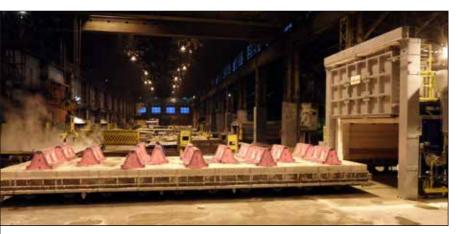
gas heated bogie hearth furnace - 51 m3 - 1200°C
