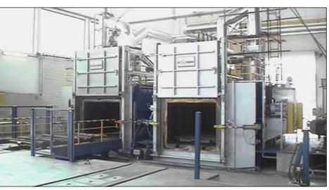
gas heated furnace - 5 tons - 550°C
