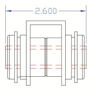
NOTE: A GAP WILL EXIST BETWEEN THE FLANGE ON THE BUSHING AND THE ARM, THIS IS BECAUSE THE STEP ON THE BUSHING IS THE STOP AND NOT THE FLANGE. DO NOT OVER-PRESS.
