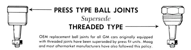
Press fit joints are slightly larger in diameter than threaded ones and are installed in the conventional manner using a T-468 press tool or its equivalent.
