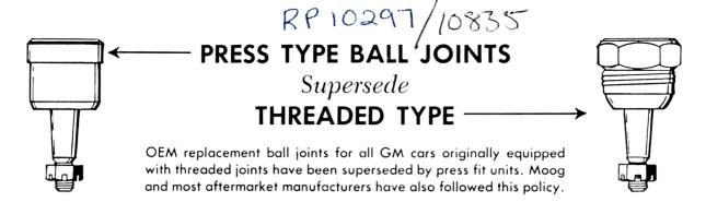
Press fit joints are slightly larger in diameter than threaded ones and are installed in the conventional manner using a T-468 press tool or its equivalent.
