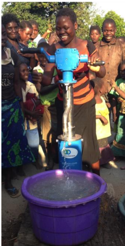
Figure 9. The first LifePump in Malawi was installed November 2013. The borehole was too deep for an Afridev and was declared dry until the LifePump arrived and could reach the water.
