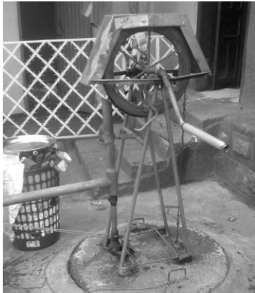
Photo 2 Typical improved Self-supply well, Ethiopia
