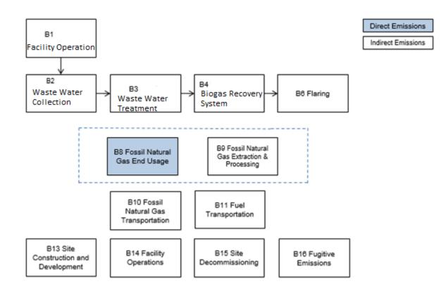
Figure 4: Project Process Flow Diagram - Anaerobic Waste Water Treatment
