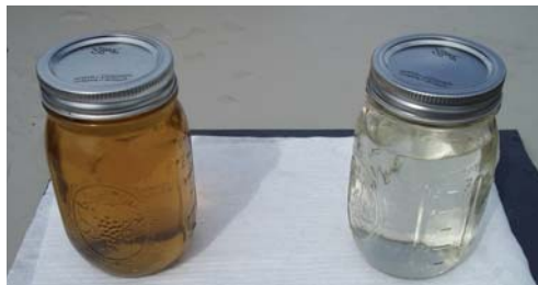
Before and After Ferrate Treatment
