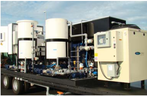
Ferrator Model Fe300 - Treats up to 90 MGD or 340,000 m 3 of water per day
