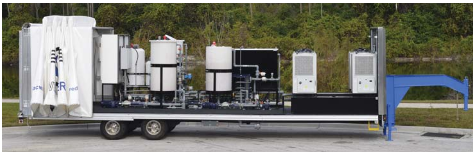
Environmental Remediation – Mobile Soft Slide Ferrator System
