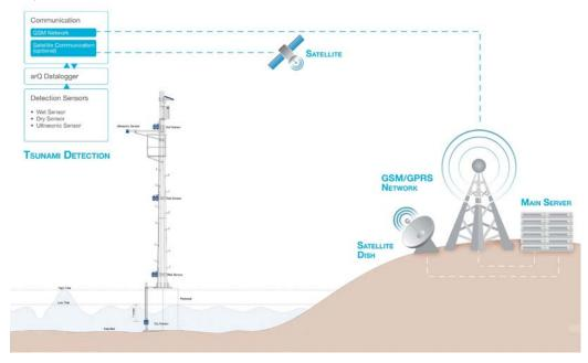
Information generated by the sensors is sent real-time to the PHIVOLCS Data Receiving Centre. If the earthquake is strong enough to be likely to cause a tsunami, the PHIVOLCS will sound off the GSM-triggered A121 Appello warning sirens to warn populations living in the affected coastal areas and give them enough time to prepare and flee their homes following designated evacuation paths leading to higher grounds (see diagram below).
