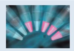
**4. Inspect tubes to determine sex** The tubes are taken out of the PCR cycler and inspected in UV light (preferably 302-312 nm, but 254 nm can also be used). Tubes fluorescing pink contain Y-chromosomal DNA. Female samples do not show fluorescence. (from left to right: F, F, M, blank, M, M, M)
