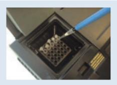
**3.** Add B-mix and run PCR The PCR program is started and 15  $\mu$ l of amplification mixture is added into each tube. The program takes about 70 minutes.
