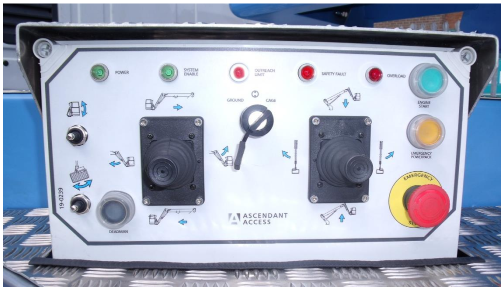
GROUND CONTROL BOX
