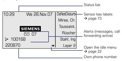
The left area contains the status bar on the first line, followed by a five-line field for additional displays. ?
