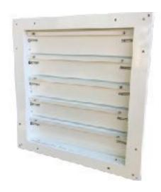
The SHX-UN BAL is an air balancing vent for use in pressurised stairwells and escape routes. They are designed to help keep an escape route balanced pressure at or below 50 pascals as is required in order for escape route doors to be manually opened in case of an emergency.
