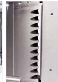
Adjustable gate flexes as top/bottom adjustable screws are turned to provide micro-adjustability of slice thickness. Sand gate limits rock and sand damage.
