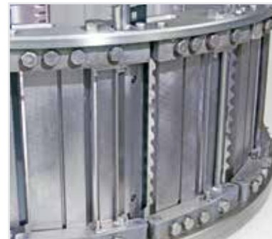
Knife holder, clamp, knife, adjustable gate, and modular block with screws makeup each of the 14 cutting stations
