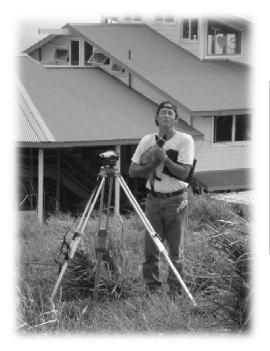
Everybody needs a Siamese survey cat! Tim is laying out the grading with approximate levels. This optical instrument he's using costs about \$400 or so and saves tons of time laying out your aquaponics system and buildings. It allows you to double-check and confirm that your grading contractor REALLY got your pads level and flat before you pay him the last payment due. It's also a great tool to use to make sure your drainage slopes drain rather than clog.
