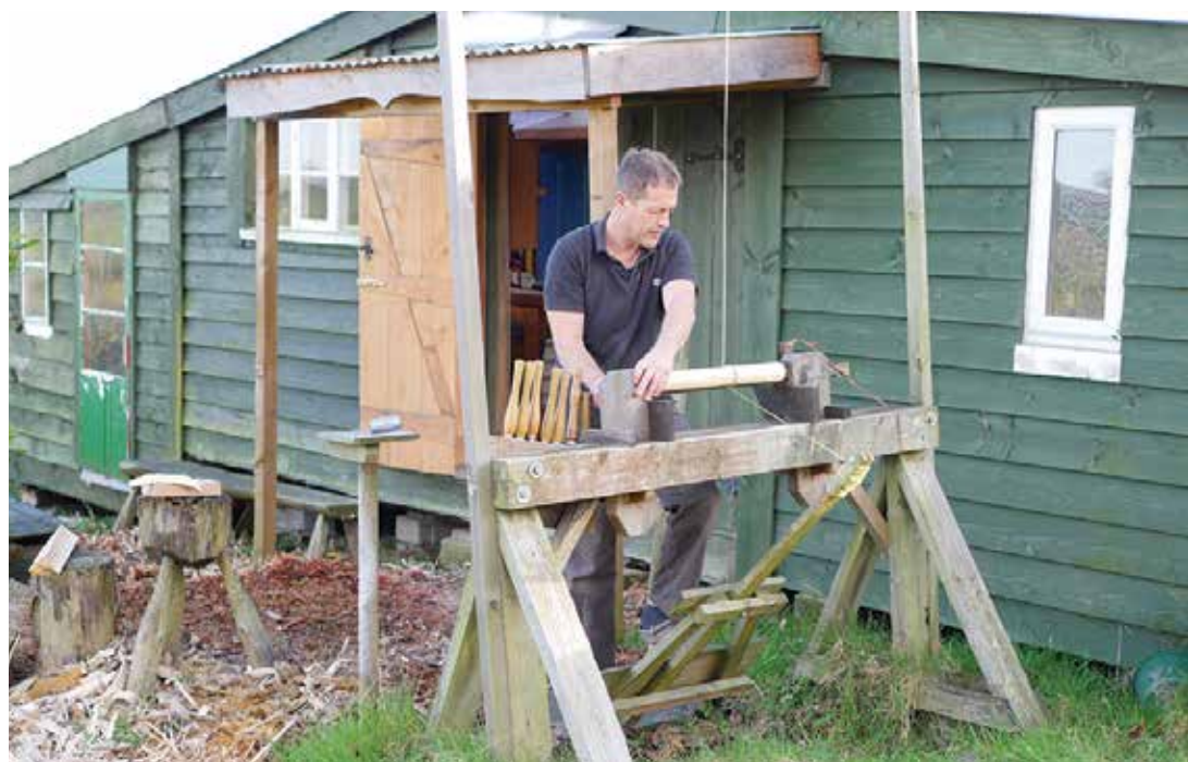
Left: David Saltmarsh on his outside pole lathe preparing to turn a chair leg. Right: Slat-back chair with cabriole legs painted with black over green milk paint.
