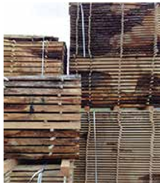
Freshly cut: boules of timber sticked and stacked for air drying at Cocking Sawmills.
